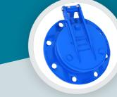
The valve has a body and bonnet in ductile cast iron EN-GJS-500-7 (GGG50) epoxy coated with 250 microns minimum thickness. The bonnet has a groove designed to fit a rubber sealing in EPDM (for water systems) or in NBR (for wastewater/sewage systems).
